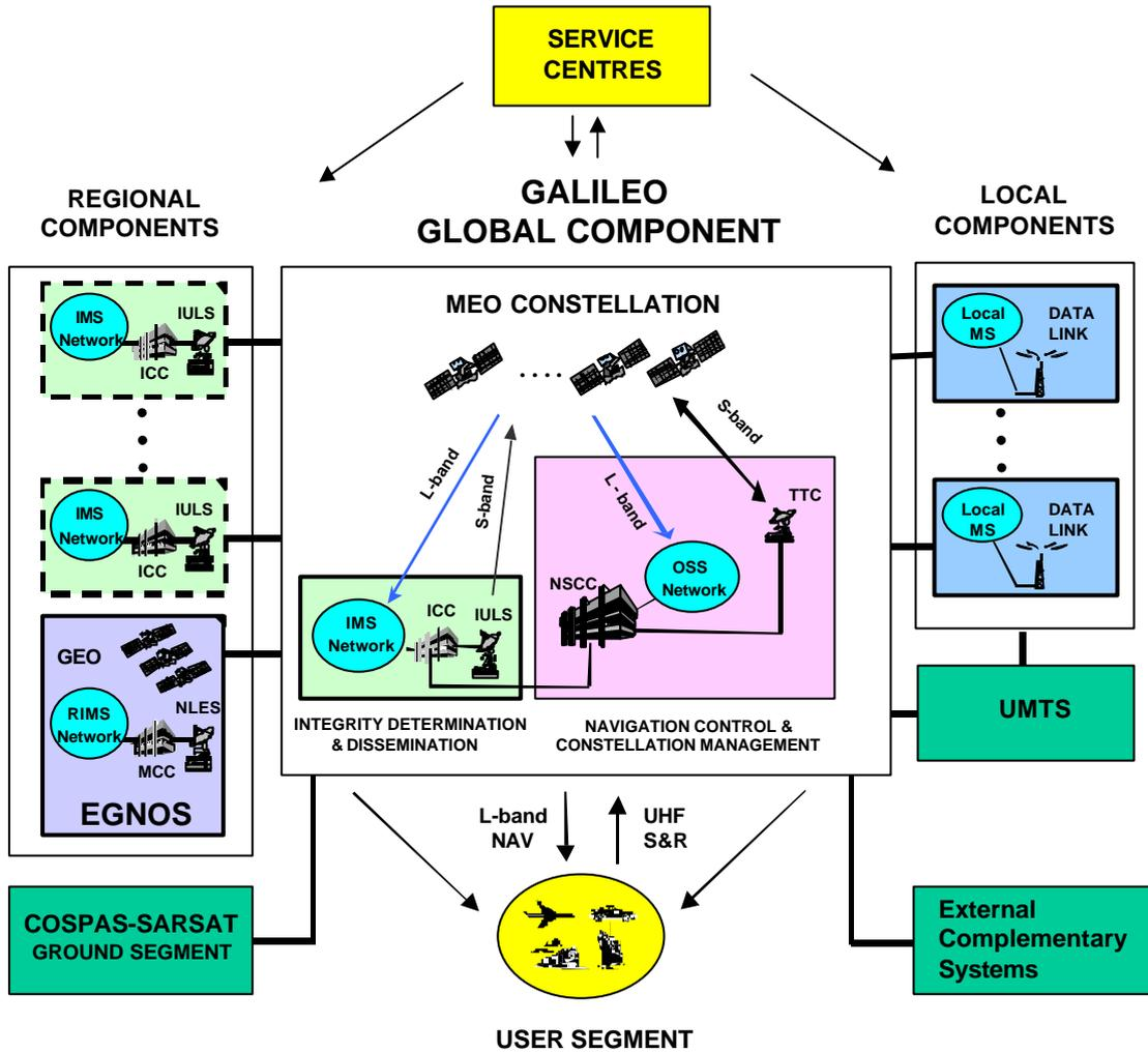
Figure 2 GALILEO Overall Architecture
